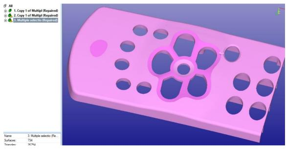
The errors are caused by some zero volume walls and intersecting triangles in them. These are created when the Offset result is added to the original model. The Offset direction follows the vertical walls of the holes in the original model:
